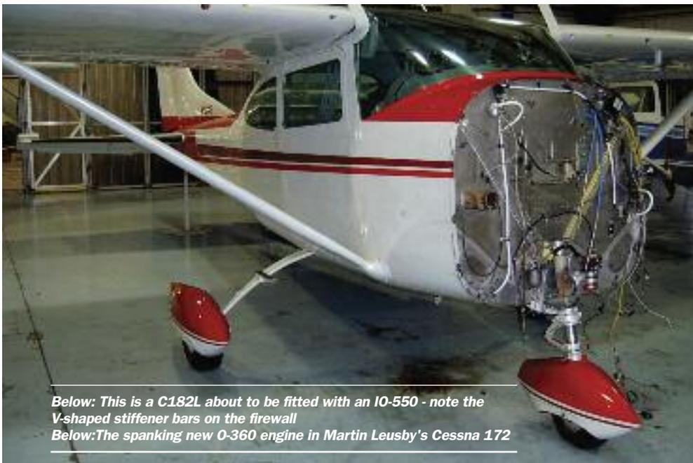
**Below: This is a C182L about to be fitted with an IO-550 - note the V-shaped stiffener bars on the firewall
