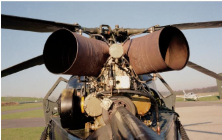
**Above: Rolls Royce Nimbus 105 engine produces 710 shaft horsepower**
