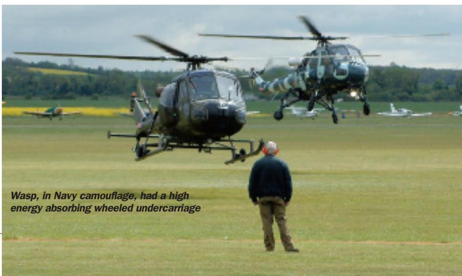
**Wasp, in Navy camouflage, had a high energy absorbing wheeled undercarriage**
