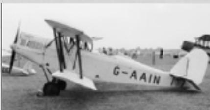
**Main photo: the layout of the Warren girder system of struts is clearly seen in this photo**
