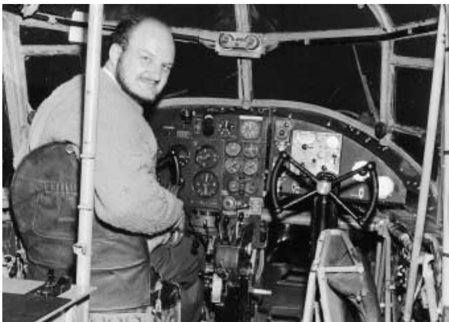
**Malcolm Payne in Anson DA. The undercarriage crank handle is to the right of the throttle levers, and the two green gear indicators are just forward, peeping from under their flaps.**
