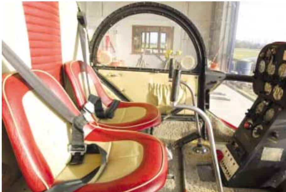
throttle takes two fingers and the response is rapid, so keeping the needle almost against the redline is a relatively simple matter. With the machine having a heavy head compared to, say, the R22, I found that rrpm changes with collective movement were small and easily matched with throttle.
