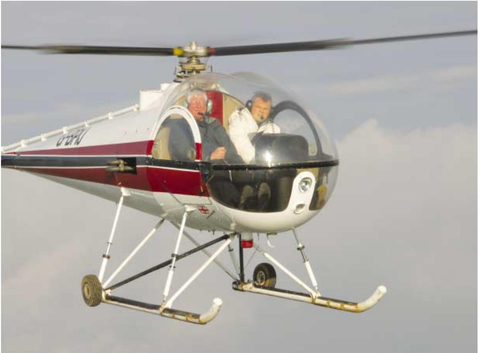
is 31 gallons, and you can lean back to 12 gph to give an endurance of more than 2.5 hr to dry tanks. Pushing the nose down and pulling back up to 25 inches brought us close to the 100mph redline, and flight remained smooth. The pitch attitude was still quite level, with none of the strap-hanging you experience with the likes of the Hiller 12 when you're three up and giving it beans. At higher power settings, however, the CHT needle soon began to threaten the redline.
