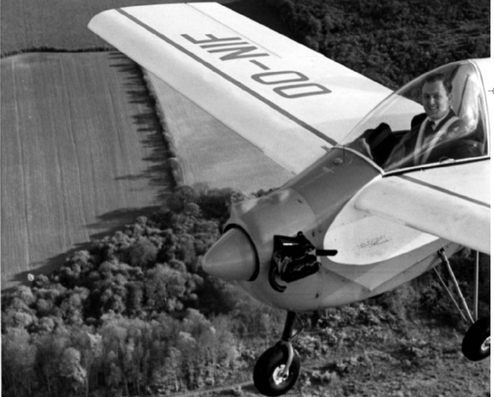
Among the Nipper's many favourable features is a good view in most directions (with downward vision panels in the wing roots) an all-flying fin/rudder, a simple undercarriage with disc brakes and an ingenious facility for accommodating a large person in a very small cockpit. The prototype took to the air late in 1957 and all early specimens were Belgian built, appearing on the market about 18 months later at a fly-away at £818.
