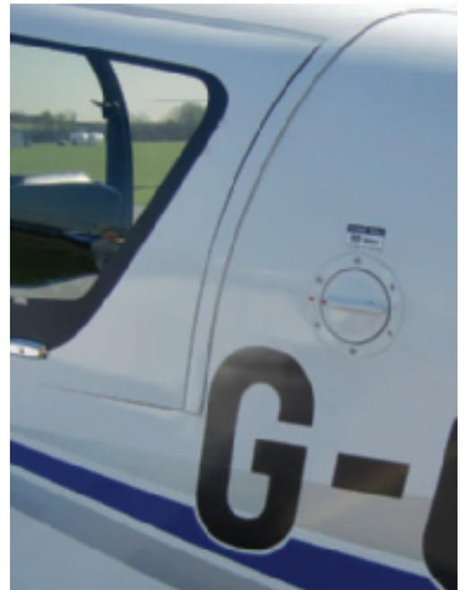
**Above right: Perspex canopy slides fully forward for ease of access**
