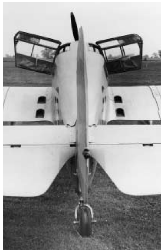
Above: rear view clearly shows the walkways on the wing centre section
