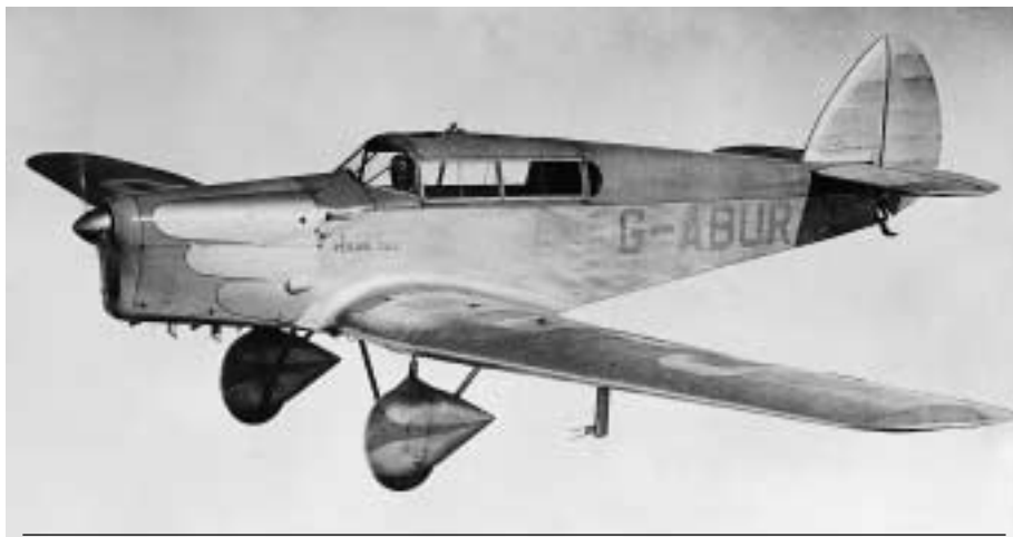
The three-seat Percival P.1 Gull Four prototype which averaged 142.37 mph in the 1932 Kings Cup Air Race powered by a Cirrus Hermes IV
