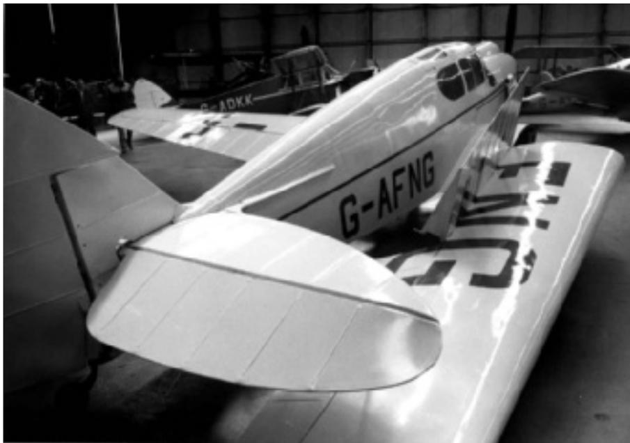
The straight stall occurs at about 45mph IAS and one wing – usually the left – goes down in an unhurried manner. With the air brake fully extended, there is no difference, which is as one would expect as, unlike a flap, it is not a lift generator; recovery is quick and easy. I did not spin her as, at the time, I had no knowledge of her recovery behaviour.
