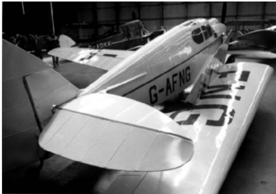
**Above: right wing root held either extra fuel tank or baggage compartment**
