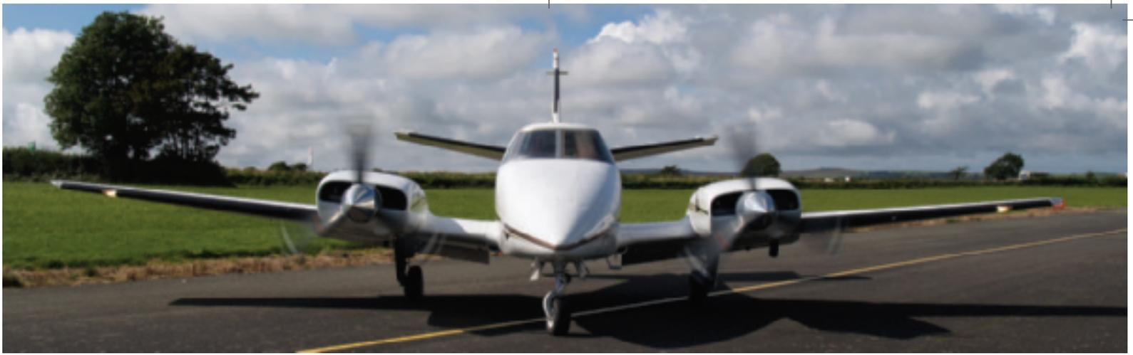
**Above: Lycomings can be replaced with P&W PT6 turboprops with 550 hp a side**
