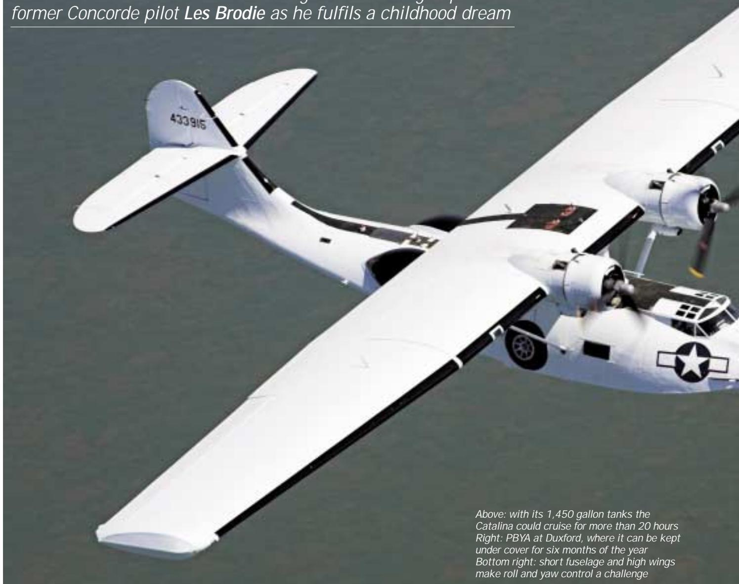
*Above: with its 1,450 gallon tanks the Catalina could cruise for more than 20 hours
