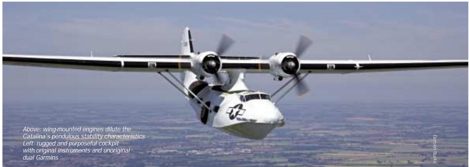
Above: wing-mounted engines dilute the Catalina's pendulous stability characteristics
