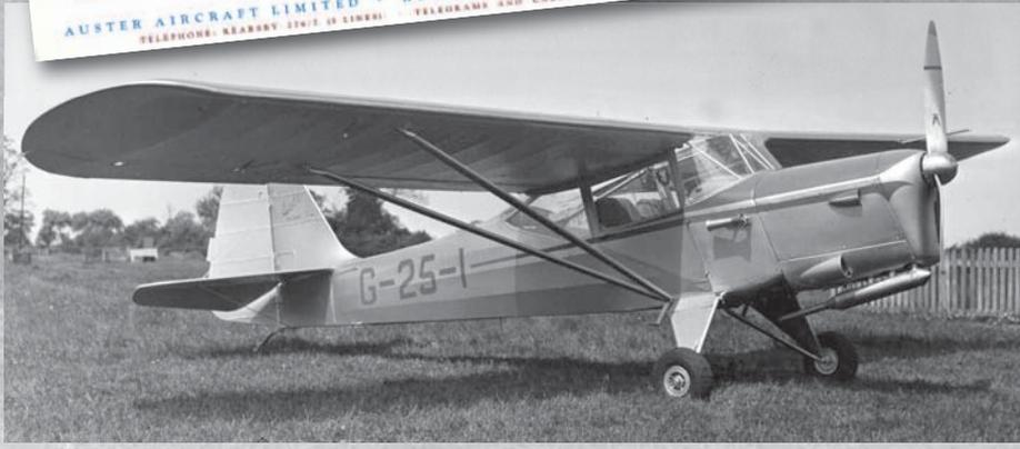
Left: the prototype Aiglet Trainer, an Autocrat fuselage married to a 130 hp engine
