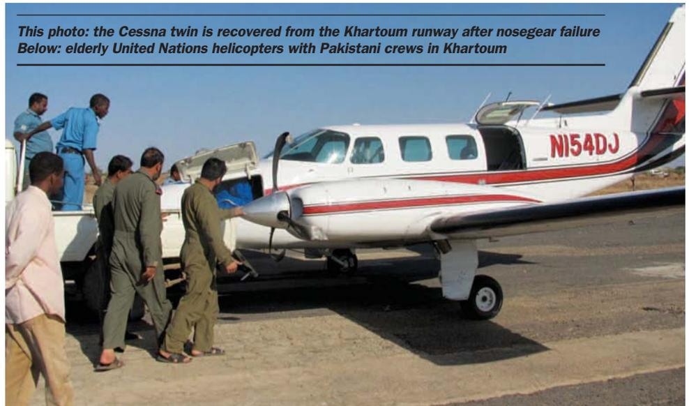
**This photo: the Cessna twin is recovered from the Khartoum runway after nosegear failure
