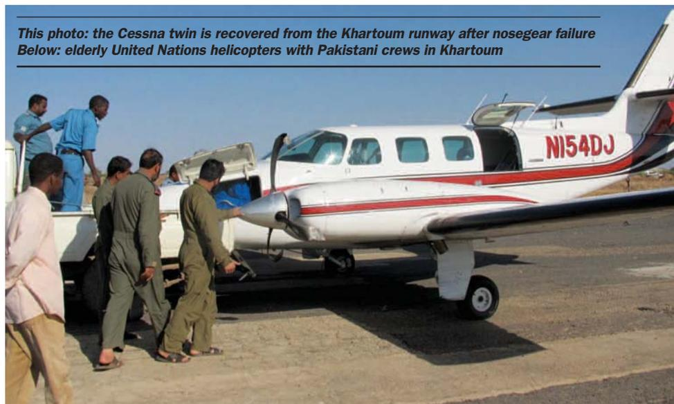
**This photo: the Cessna twin is recovered from the Khartoum runway after nosegear failure
