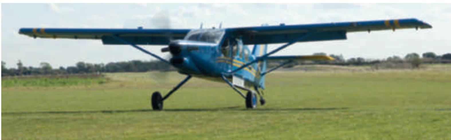
burning about 150 kg (187 litres) of Jet fuel an hour in this configuration.
