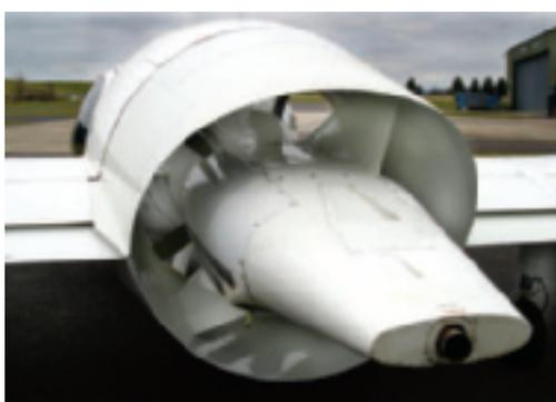
and main spar. Although a pusher propeller could have been mounted high above a more conventional structure, the duct design has several advantages: it allows the engine thrust to be closer to the aerodynamic thrust line giving better stability with power changes, it protects the propeller from ground strikes, it's quieter than a conventional prop, and the duct gives better performance at slow speeds. Plus, "ducts were in fashion at the time" Edgley said in an interview.
