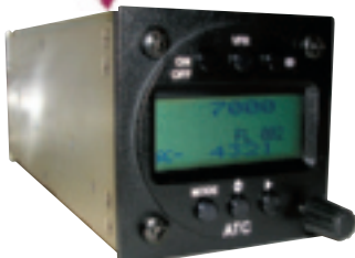
TRT 800 Transponder Modes A/C and S. Integral alticoder. Easy installation
