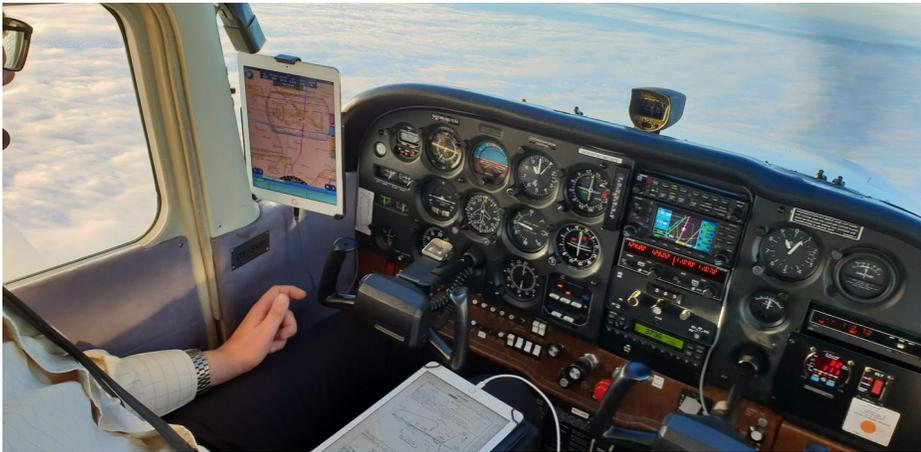
The following pictures are from a Cessna 172 where two ipads are used. One is mounted on a knee-board and the other with a RAM suction cup mount. The charging cable for the latter is a quality cable sufficiently long that it can follow the curve of the dashboard all the way around so it does not interfere with any controls or handles.
