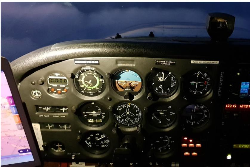
A special advantage of this mounting location is that the flashlight on the back of the ipad can be used as a backup lightsource should the electric power of the aircraft disappear. It can be a good idea to switch on the light before it becomes dark. Then you are prepared and don't suddenly need to
