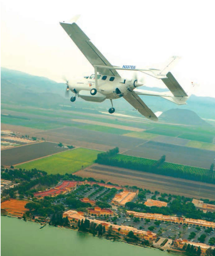
1 Ampaire's hybrid-electric testbed – the EEL is a converted Cessna 337 Skymaster
