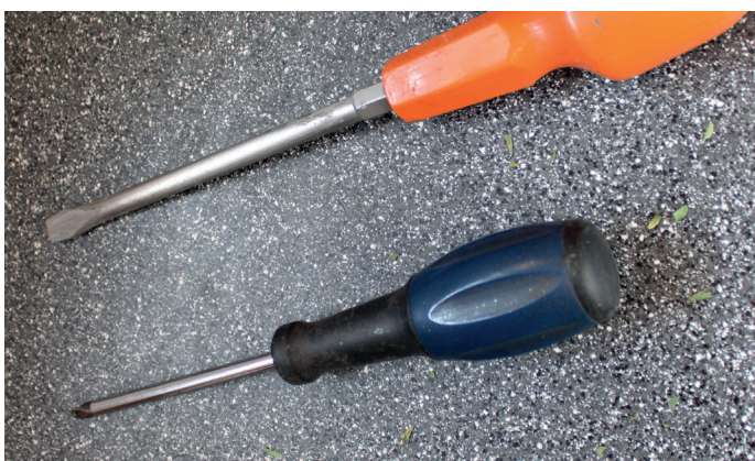
Over time, a worn screwdriver will begin to damage screws
