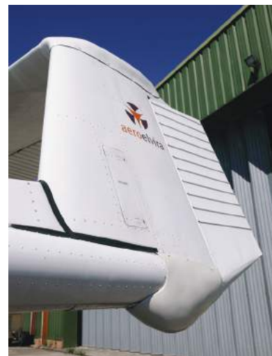
The ballast weight door in the starboard fin.
