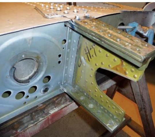
**Left: having to remove wings for inspection on older Cessnas would effectively write them off
