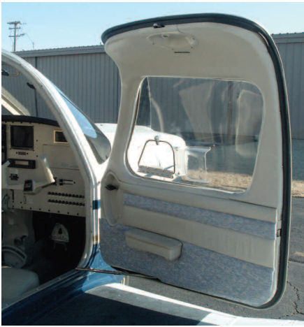
Left: Swedish interpretation of Part M means door seals must be lubricated every 30 days, which is causing safety problems
