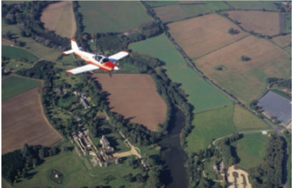
Top: take-off requires less than half of a 650 metre grass strip Above: in the cruise at 24 squared, the Monsun burns about 28 litres per hour Below: 'a strong, controllable two-seater with adequate range'
