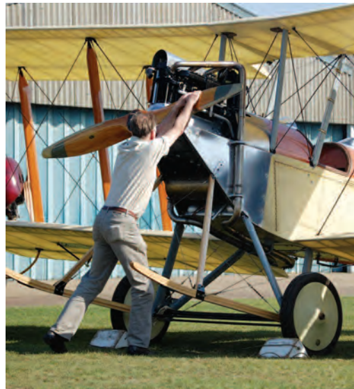
Above: BE-2 panel – modern oil pressure gauge (bottom right) is a temporary fixture Left: starter takes care not to loop fingers over the trailing edge for fear of kick-back This photo: the aircraft's crosswind tolerance is limited – to zero
