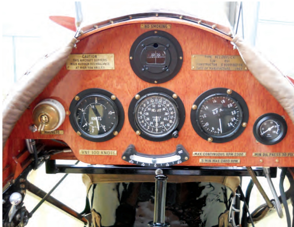
Above: BE-2 panel – modern oil pressure gauge (bottom right) is a temporary fixture Left: starter takes care not to loop fingers over the trailing edge for fear of kick-back This photo: the aircraft's crosswind tolerance is limited – to zero
