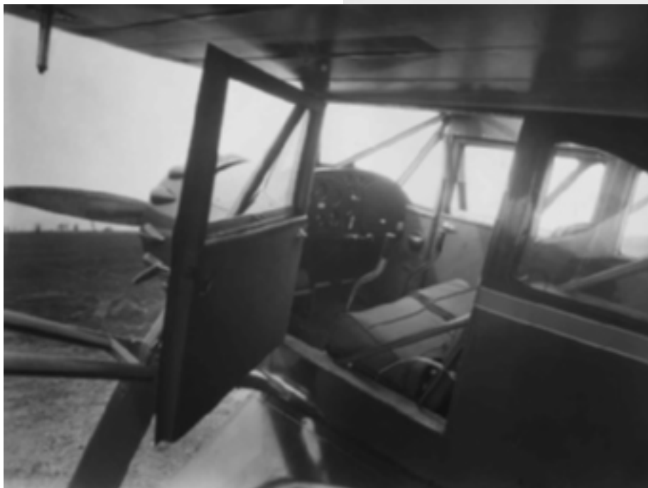
Above: Ranger-engined version was not approved in the UK until after the war Left: car-type doors gave access to a relatively spacious cockpit
