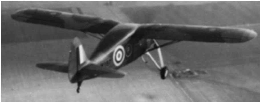
This photo: in calm conditions the F24 could be flown hands- and feet-off Below: parasol wing helped to give the Argus an unusual degree of stability
