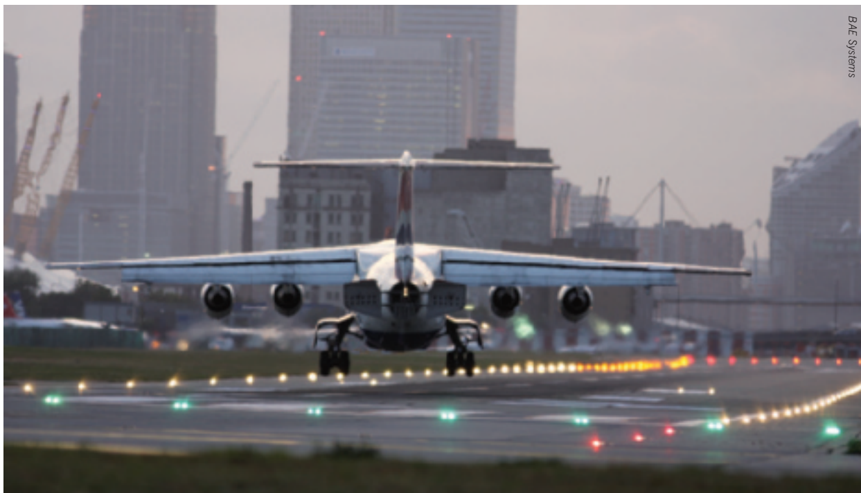
Left: don't straighten up before touching down after a crab approach – the plane weathercocks perfectly well around the first bogey to touch, and it's more important to maintain the centreline
