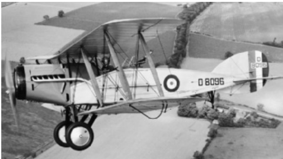
Top: Hucks starter was an alternative to the armstrong method Above: this angle shows how the fuselage lies midway between the upper and lower wings Below: B2bs of 141 Sqn at Biggin Hill, late 1918. Note four-bladed props
