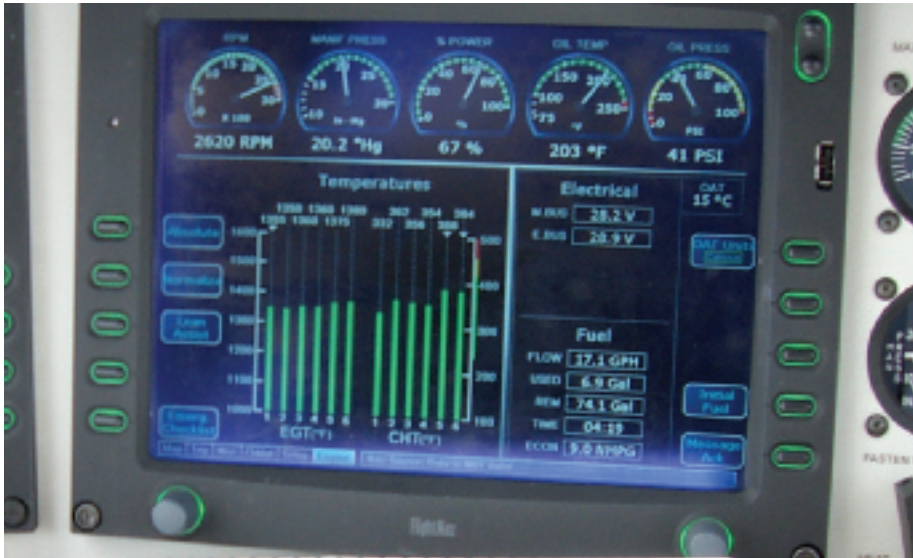
Right: engine page shows EGTs and CHTs for all cylinders, together with fuel flow and much more
