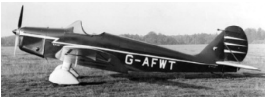
Above: the large single-piece protective windscreen is clear to see; in balanced flight it is very effective
