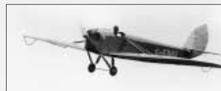
Above: note the DH51's unusual tailskid and the large G on the rudder - mandatory on all British civil aircraft until 1928 Below: the diminutive DH53
