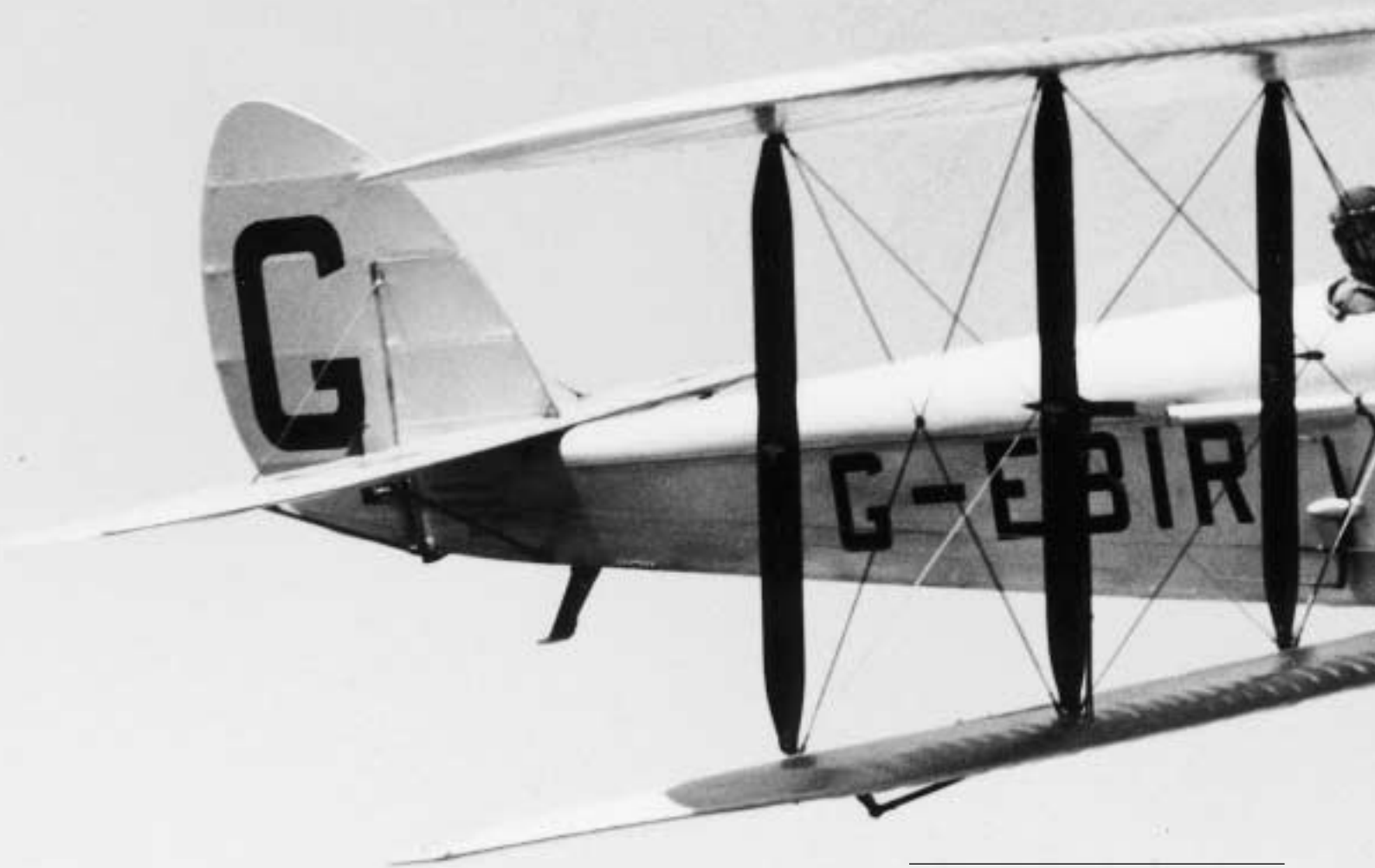
Above: note the DH51's unusual tailskid and the large G on the rudder - mandatory on all British civil aircraft until 1928 Below: the diminutive DH53
