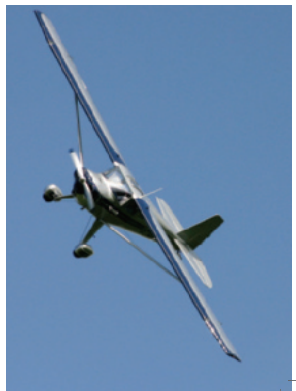
Left: Model 8E has all-metal wing and wing tanks. Note single lift strut and rear cabin windows. Above: 8A has fabric covered wings, two lift struts and fuselage tank, hence no rear cabin windows. Both have the earlier main gear with bracing wires Below: cosy cabin - similar in size to a 152 - and a view of the relatively high aspect-ratio wing
