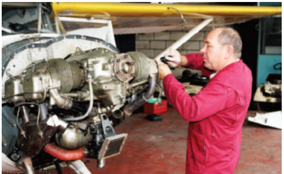
Above and right: adjusting the brakes; the later Sillflex gear with fairings removed. Floorboards out for the annual, rudder cables in centre. Robin replacing a rocker cover on the mighty C85
