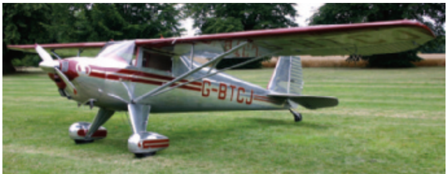
Left: Model 8E has all-metal wing and wing tanks. Note single lift strut and rear cabin windows. Above: 8A has fabric covered wings, two lift struts and fuselage tank, hence no rear cabin windows. Both have the earlier main gear with bracing wires Below: cosy cabin - similar in size to a 152 - and a view of the relatively high aspect-ratio wing
