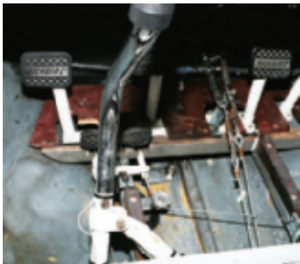
Above and right: adjusting the brakes; the later Sillflex gear with fairings removed. Floorboards out for the annual, rudder cables in centre. Robin replacing a rocker cover on the mighty C85
