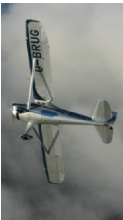
Left: Model 8E has all-metal wing and wing tanks. Note single lift strut and rear cabin windows. Above: 8A has fabric covered wings, two lift struts and fuselage tank, hence no rear cabin windows. Both have the earlier main gear with bracing wires Below: cosy cabin - similar in size to a 152 - and a view of the relatively high aspect-ratio wing
