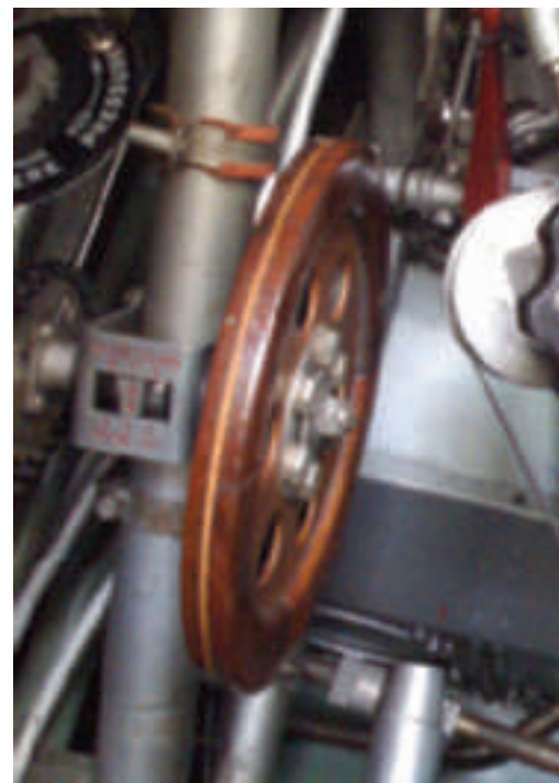
Above: the Hurricane's cockpit is very deep and rearward view is poor Left: undercarriage and flap lever might have been designed to cause maximum confusion Below: the beautifully-crafted mahogany trim wheel speaks of a different era Right: if it looks right it'll fly right, as Sir Sydney Camm used to say Bottom right: star-shaped rudder trim and pneumatic pressure gauge
