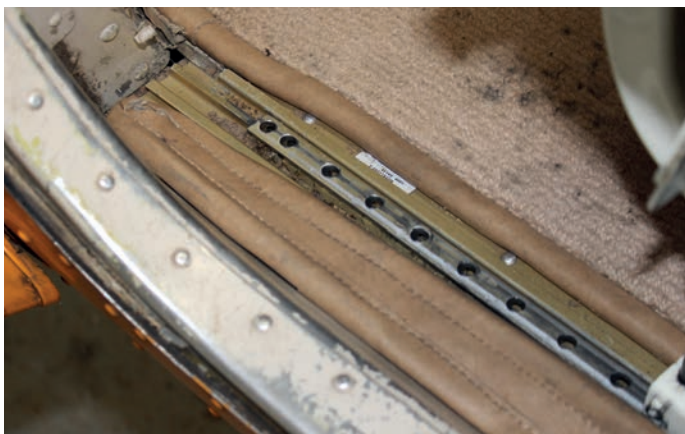
Check the rivets to see if there's any movement
