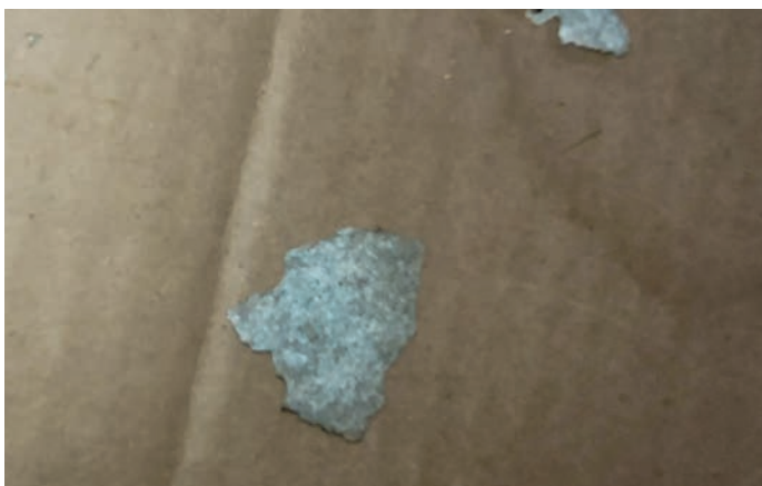
Chips of corrosion from the airframe
