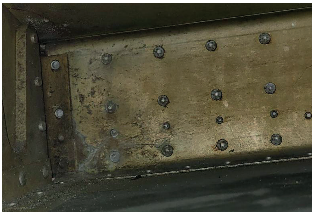
If you spot corrosion before it takes hold of your airframe, you could save a lot of money
