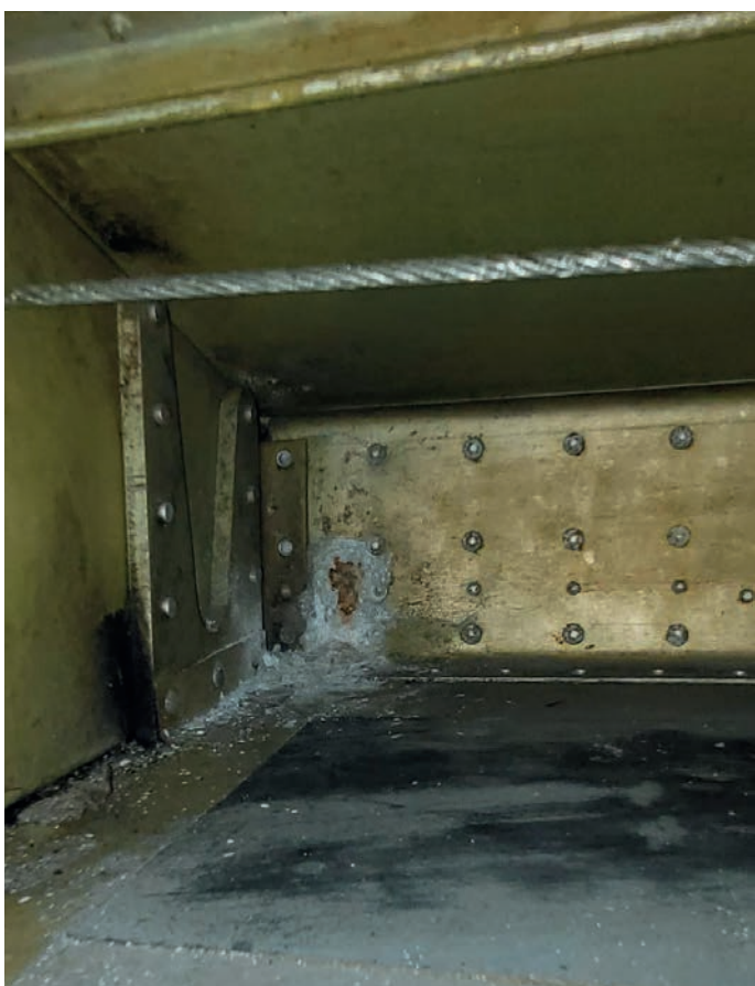
Corrosion spots inside a PA28, which can be a familiar sight
