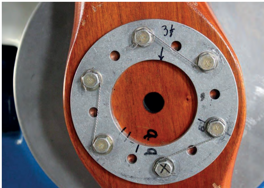
The wire-locking must counter the direction used to remove a bolt, nut or item such as a filter
