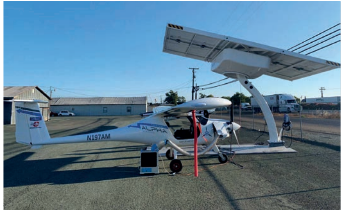
The Beam Global Pipistrel Alpha Electro is charged using Beam's solar-powered charging equipment.
