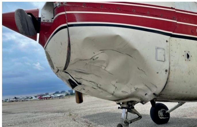
This is what happens when a drone hits a Cessna. Imagine what would have happened if it had been a few feet higher.
