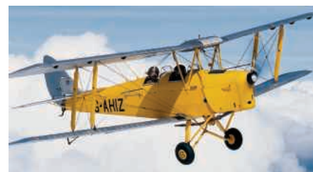
Below: Moth's tailskid turns with the rudder to aid ground handling Right: you can learn to fly the Tiger Moth with Cambridge Flying Group
