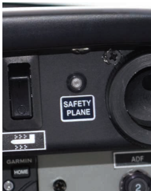
Left: 'Safety Plane' stores exceedence data for engineers and flight schools Right: stick has been redesigned, simplified and cleaned up Below: flying characteristics are very similar to those of the Robin DR400 Bottom: fully loaded the DR401 can break ground in just over 170 metres
