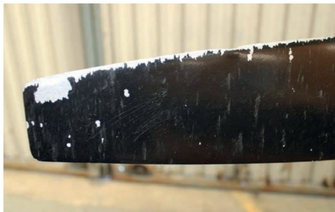
Figure One: Spot the dent in the leading edge, caused by a stone. This could be enough to make it unrepairable
