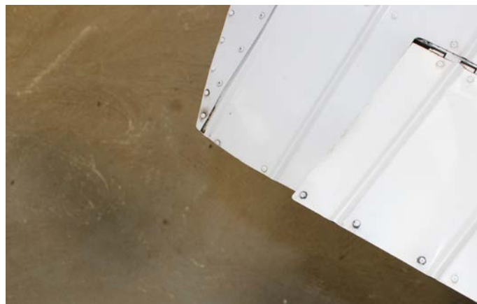
Figure Two: Beware of 'smoking' rivets, the grey or black markings around a rivet head are caused by the loose rivet
