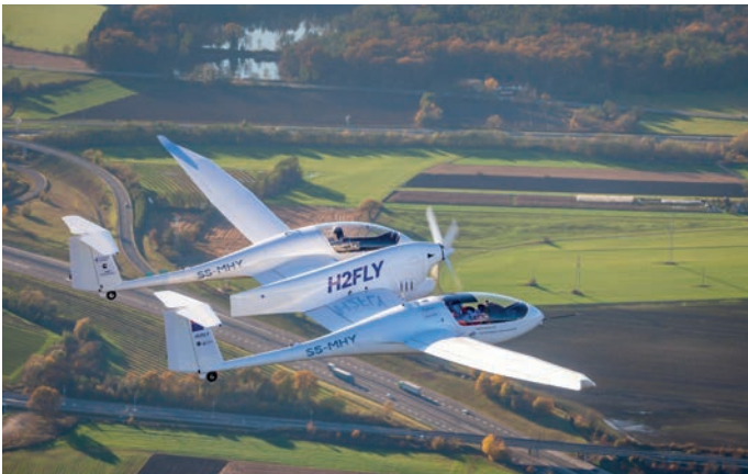
German company H2FLY's, the HY4, an aircraft that flew to Friedrichshafen with zero emissions using green hydrogen
