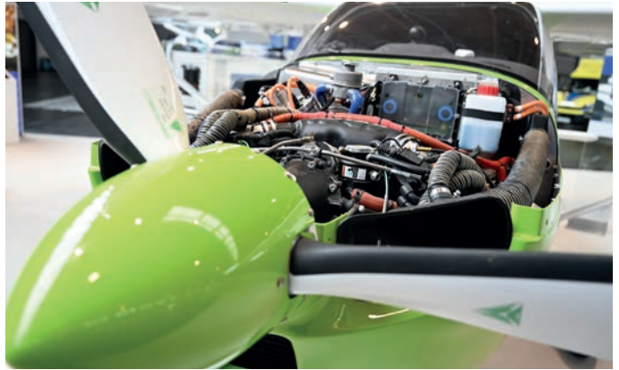
An electric motor connects to the crankshaft to provide a power boost for take-off and start the P2010 H3PS's engine
