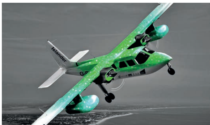
The Scottish Hydrogen Fuel Tank (SHyFT) system will carry the gas beneath the wings of the Project Fresson Islander.
