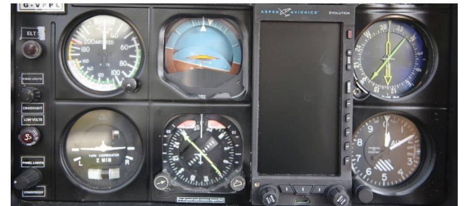
The 'Basic Six' panel. The main Instruments Rule could be said to be that you either are VFR or IFR. On this panel you also have the option of using the glass panel.
