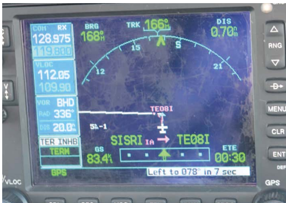
Bottom right: the green LPV flag at lower left comes up with 2nm to run to the final approach fix
