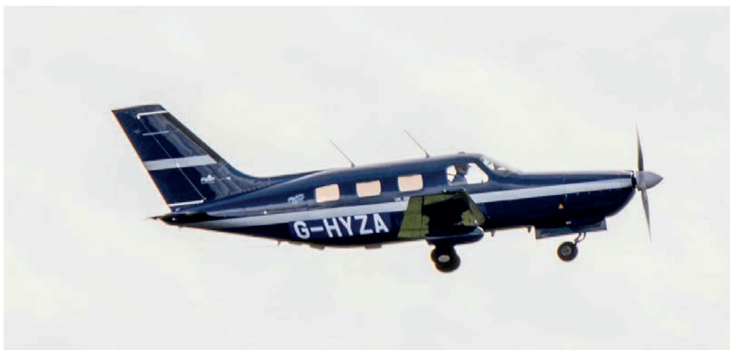
The ZeroAvia Malibu was the first commercial-grade hydrogen-electric aircraft to fly. Funding has been granted to develop a 19-seat aircraft by early 2023.
