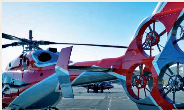
The Bell 427 demonstrator drives the four motors using dedicated generators in its Pratt & Whitney turbines.
