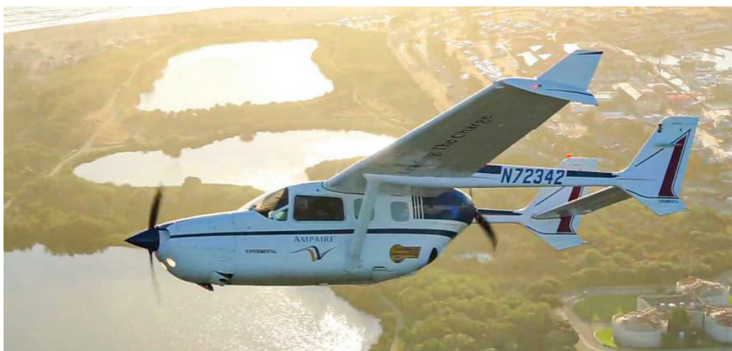
The Electric EEL is a converted Cessna 337 Skymaster powered by a rear-mounted 310 hp Continental IO-550 engine and a 160 kW (119 hp) electric power unit in the nose.
