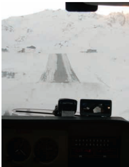
Far left: on long final for 22 an escape would be possible with a steep turn to the right Left: all go-round options lapse a long way out, and a landing must be attempted Above: on touchdown, full power must be applied to make sure the aircraft can reach the apron
