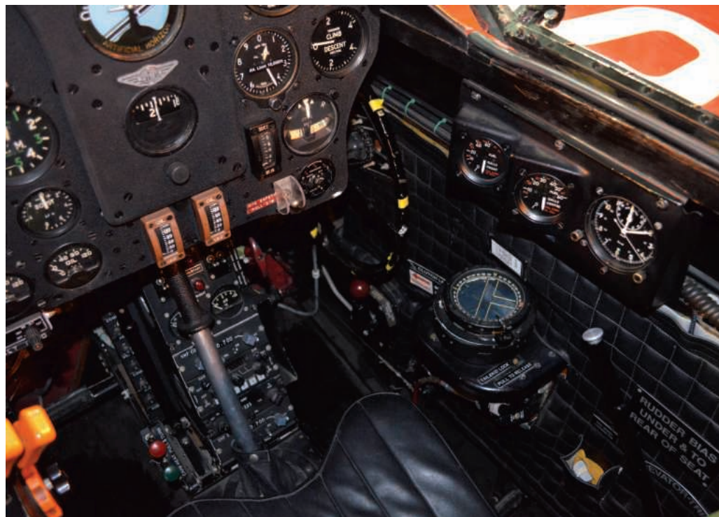
Left: Dodge Bailey checks the Comet's undercarriage, originally a design weak point Above: the CHT gauges atop the coaming provide pitch clues on take-off and landing Right: the two plungers with which the ground crew prime each Gipsy engine Lower left: mixture, prop and throttle controls – the silver knob is the flap lever Below: crossfeed cock, P-type compass, tailskid lock – yellow-striped wheel is manual undercarriage
