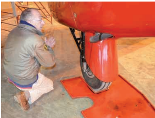
Left: Dodge Bailey checks the Comet's undercarriage, originally a design weak point Above: the CHT gauges atop the coaming provide pitch clues on take-off and landing Right: the two plungers with which the ground crew prime each Gipsy engine Lower left: mixture, prop and throttle controls – the silver knob is the flap lever Below: crossfeed cock, P-type compass, tailskid lock – yellow-striped wheel is manual undercarriage
