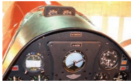
Left: Dodge Bailey checks the Comet's undercarriage, originally a design weak point Above: the CHT gauges atop the coaming provide pitch clues on take-off and landing Right: the two plungers with which the ground crew prime each Gipsy engine Lower left: mixture, prop and throttle controls – the silver knob is the flap lever Below: crossfeed cock, P-type compass, tailskid lock – yellow-striped wheel is manual undercarriage
