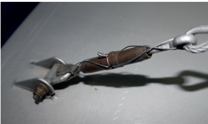
Note how the turnbuckle is wire-locked before undoing it
