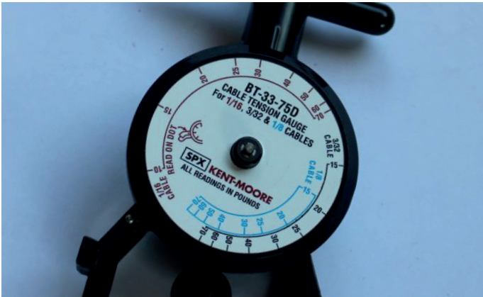
Fig 1: Cable tensiometers are a good way to check cables
