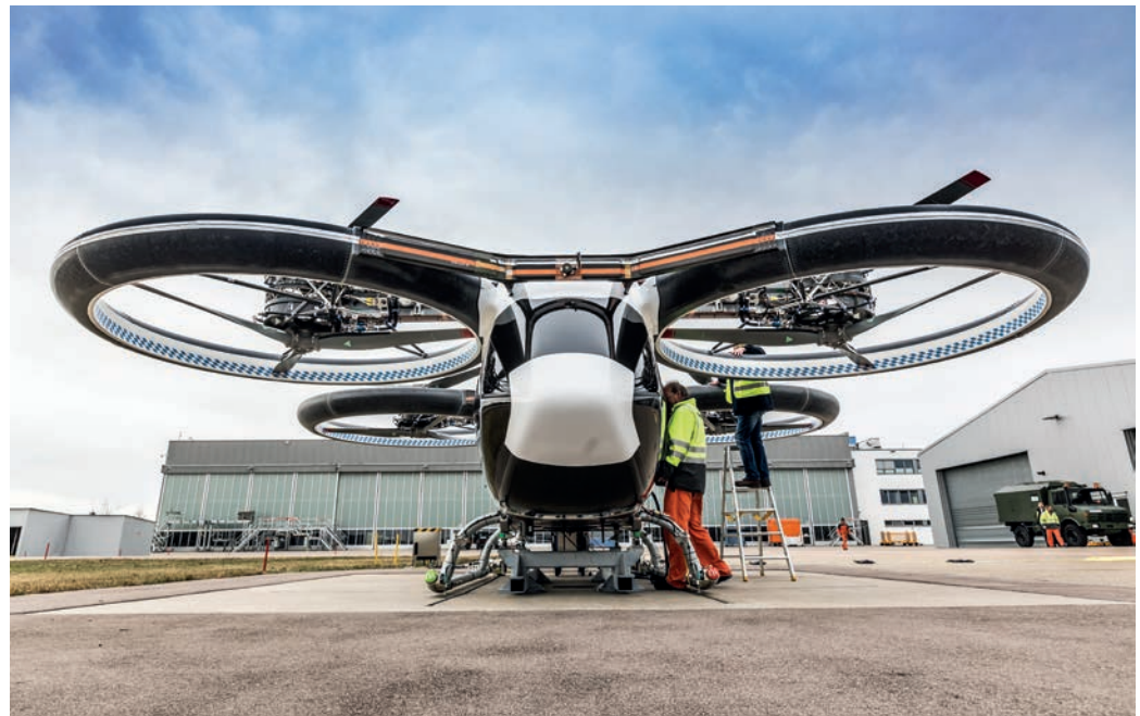
The CityAirbus NextGen is an all-electric, four-seat multicopter concept featuring a wing
