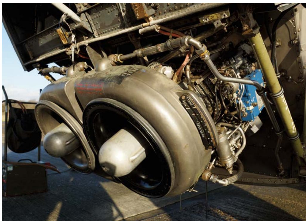
This photo: all aboard the FunBus... the Wessex hovers out of dispersal at Biggin Hill Below: Coupled 1350hp Bristol Siddeley (later Rolls Royce) Gnome turbines made it go
