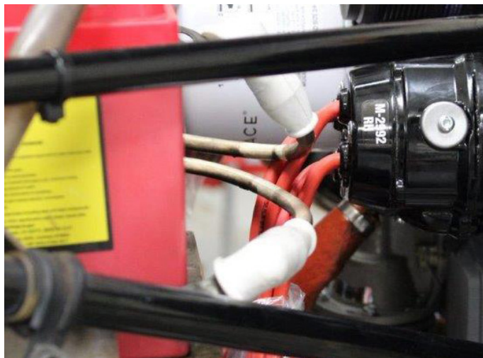
The oil filter can be cleaned in Avgas and checked for fragments
