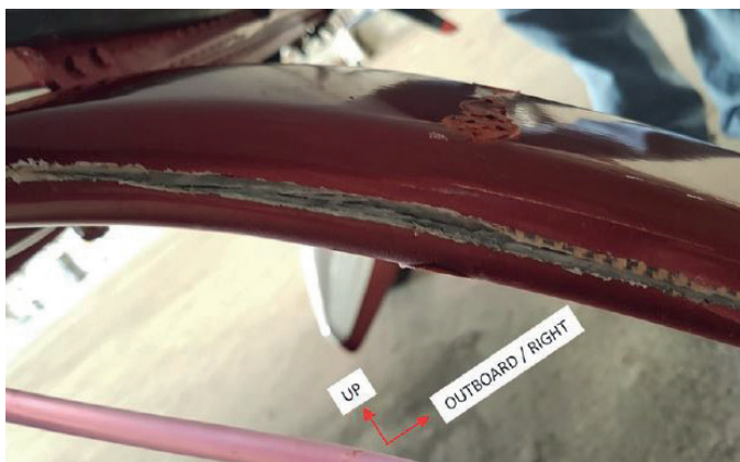
The crack along the undercarriage leg was noticed after landing and the aircraft immediately grounded
