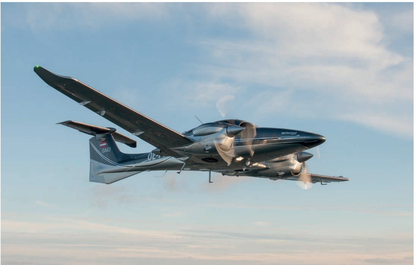
The state-of-the-art carbon fibre composite airframe makes this twin lighter than most
